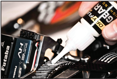
Gear Lube benefits in reducing friction and wear on main gears and pinions
