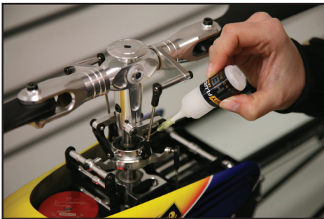
Dryfluid besides lubricating it leaves a small anti dust film on the parts where we apply the product
